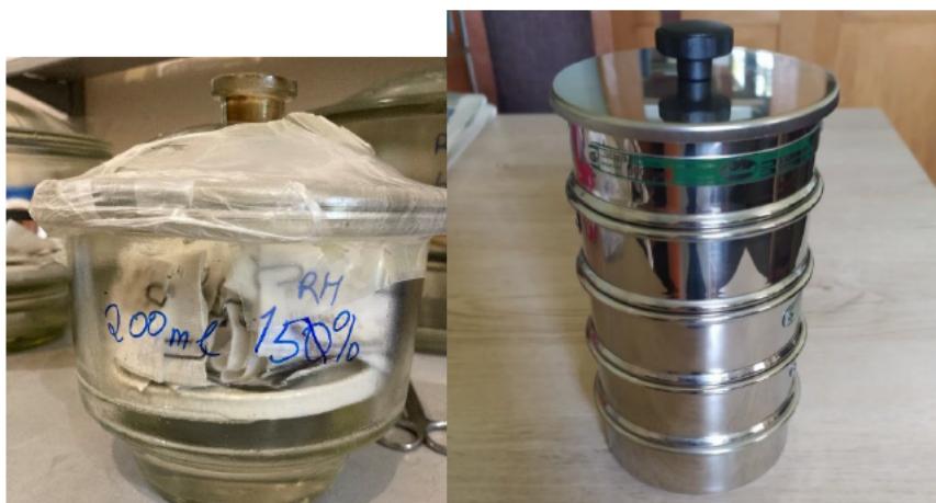
Figure 10: Drying chamber (left) and new fine sieves (right) for orchid processing and precision drying.
